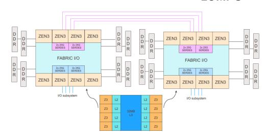
2x 64-core AMD Milan processors per node 1376 nodes with 256 GB, 128 with 512 GB and 32 with 1 TB
